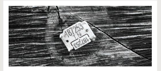
Once the tree has been bought at auction it is cut into large wood boards. Those will then stay in the open air, under the rain and sun for 3 years in order to eliminate the green tannins and to reinforce the durability of the wood over time.
